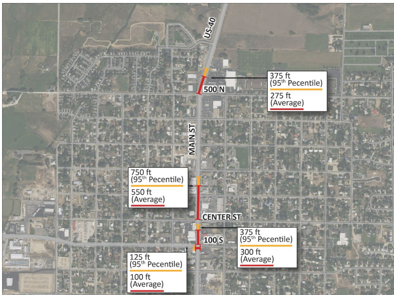
Figure 8. Vehicle Queue Lengths at Key Intersections in the Needs Assessment Evaluation Area during the Current PM Peak Hour
