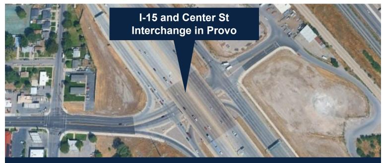
A tight diamond interchange features closely spaced, signalized intersections where freeway ramps meet the cross road to minimize the footprint.
